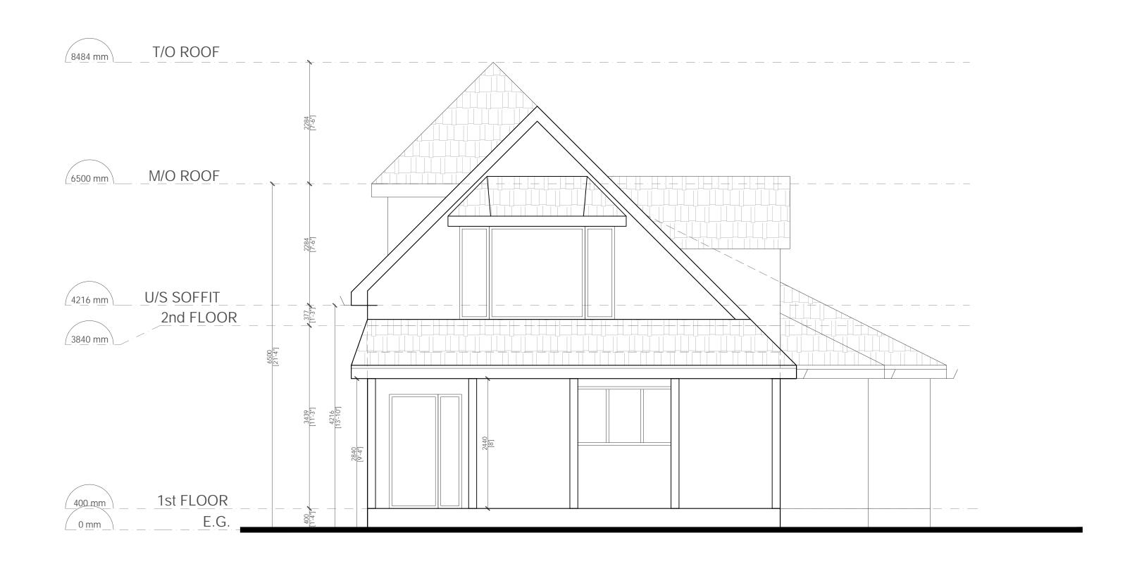
1 EXISTING FRONT ELEVATION A304 SCALE: 1:50
