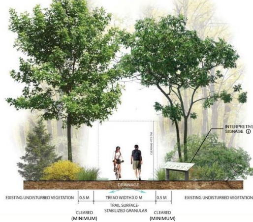
Figure 34: Typical Granular Nature Trail Cross Section
