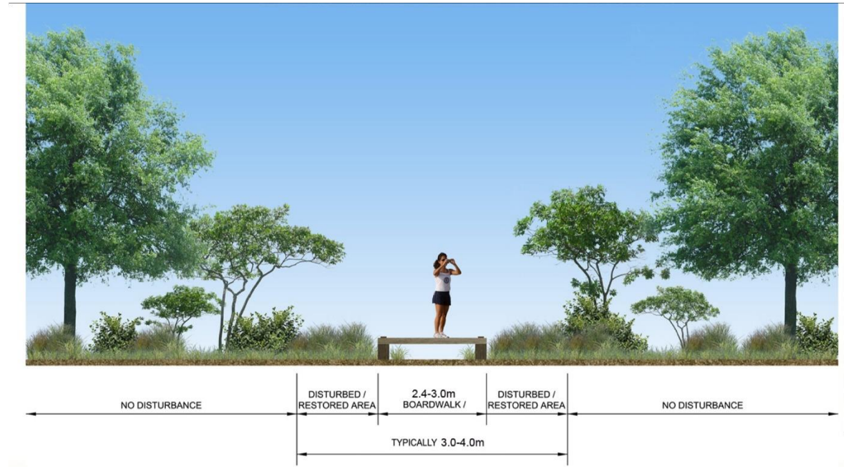
Figure 32: Typical Boardwalk Cross Section
