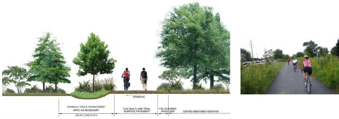
Figure 35: Typical Asphalt Multi-Use Trail Cross Section
