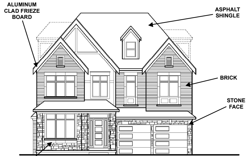
FRONT ELEVATION - FACING INTERIOR ROAD
