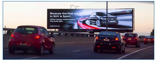
**Power Requirements:** 32 Amps **Brightness\*:** 8,500 nits when shipped; 5,000 nits at year 10 guarantee **Service Access:** Front and rear access-standard **Environmental Protection:** Fully-sealed IP-67 module, fully-sealed power supply, and PLR **LEDs per Pixel:** 3 color matched LEDs: 1 red, 1 green, 1 blue **Viewing Angle:** 160° H x 70° V **Compliance Information:** UL, cUL, UL-Energy Verified, IBC 2012, FCC Compliant **Operating Temperature:** -30° to +120° F (-34° to +49° C)
