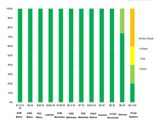
Figure 5-3: Asset Condition Detail (Stormwater Services)
