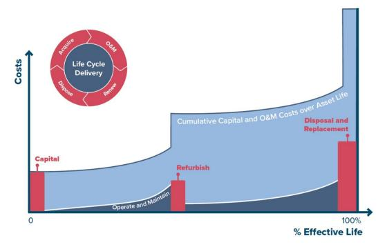
Figure 2-3: Life Cycle Cost Accumulation Over Asset Life
