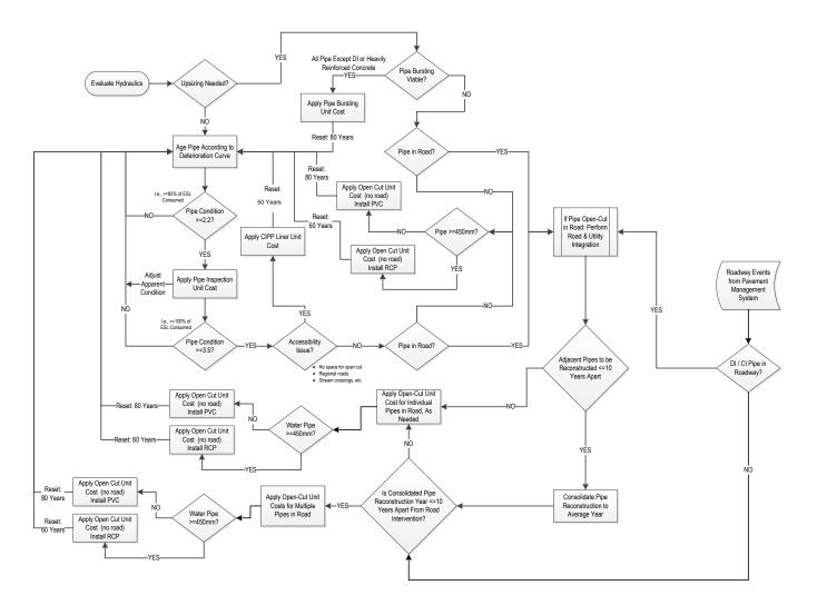
Figure 3-6: Water Process Flow
