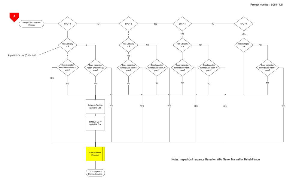
Figure 4-6: CCTV Process Flow
