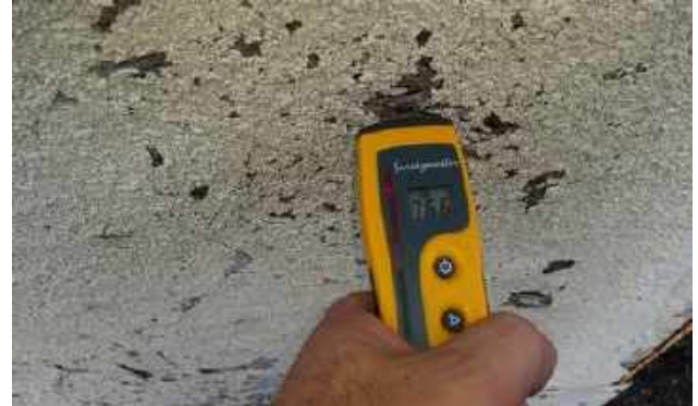
Water saturated stucco wall
