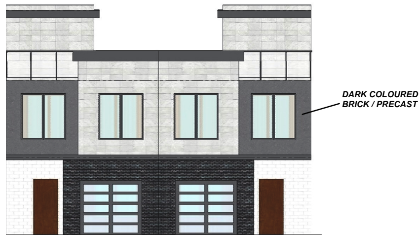
FRONT ELEVATION (BLOCK 7: SEMI-DETACHED TOWNHOUSES) - FACING PRIVATE LANEWAY (3-STOREYS)
