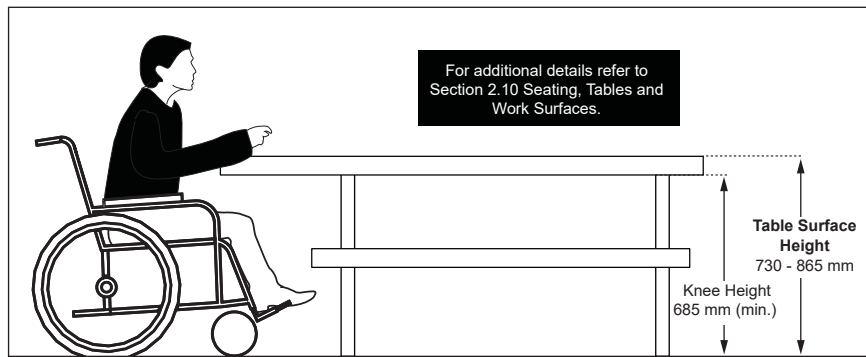
Figure 101b: Picnic Table Design and Features - Elevation View
