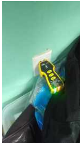
Reverse polarity condition
