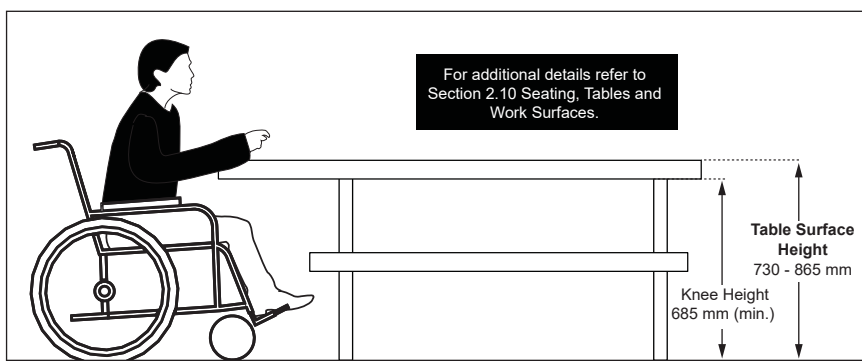
Figure 101b: Picnic Table Design and Features - Elevation View
