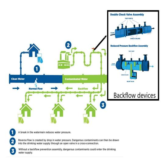
Figure 1- Graphical illustration of how the Backflow Prevention Device works
