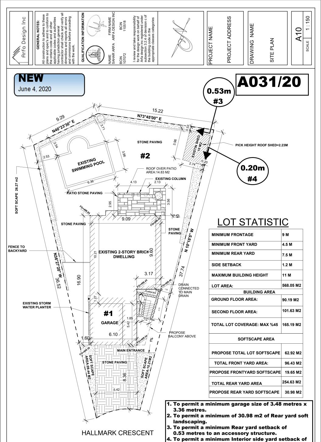
ALL AREA ARE STONED PAVING EXCEPT THE DOTET HATCH THAT REPRESENT THE SOFT SCAPING
