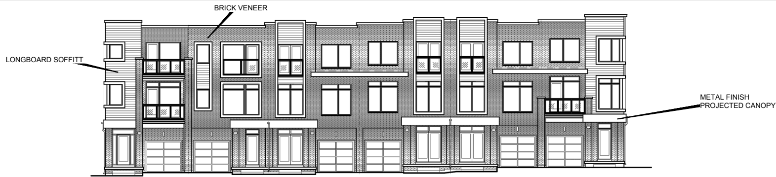
FRONT ELEVATION (FACING INTERNAL ROAD)
