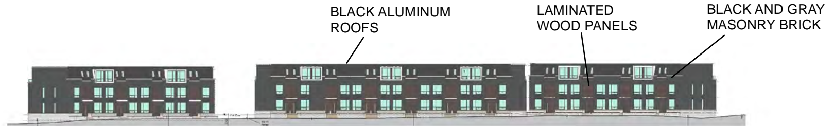
BLOCKS C, D AND E - WEST ELEVATION (FACING INTERNAL PRIVATE ROAD)
