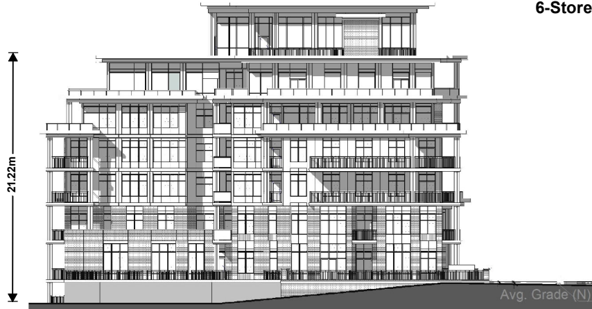
North Elevation - Building N
