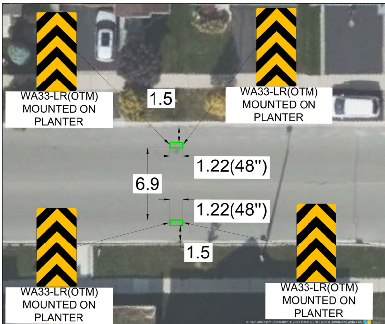
Figure 4: Design Example of Planters Aligned
