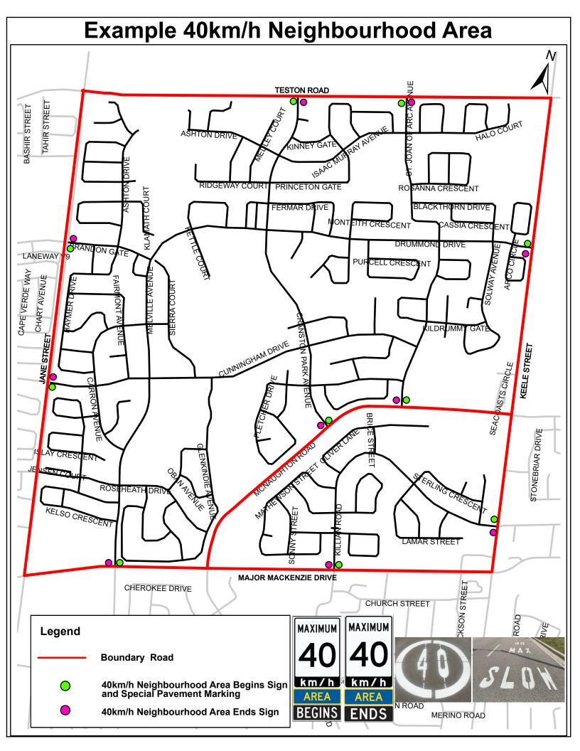
Example Signage and Pavement Marking in road set up
