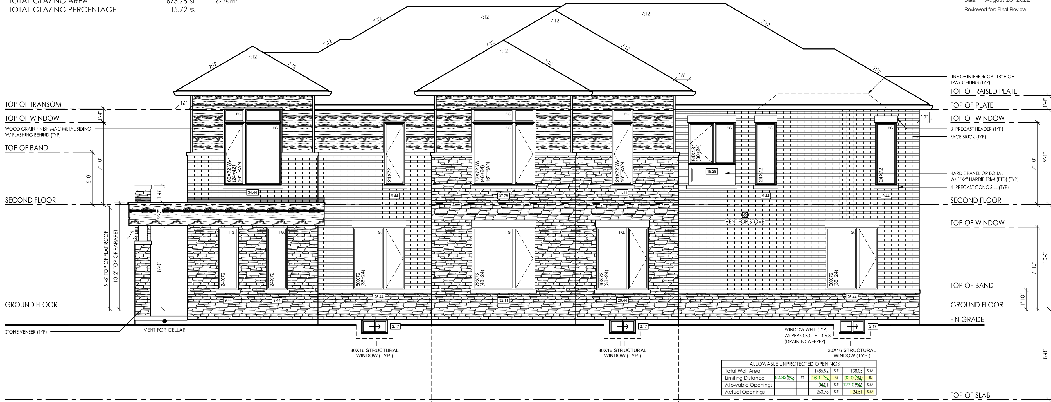
UPGRADED RIGHT SIDE ELEVATION 'B'
