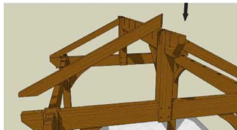
QUEEN RAFTER/KING POST CONNECTION (DOVETAIL CONNECTION) N.T.S.
