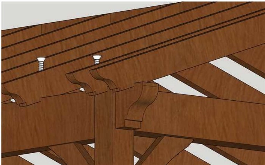
SUPPORT BEAM/RAFTER CONNECTION N.T.S. (11" timber screw for additional reinforcement)
