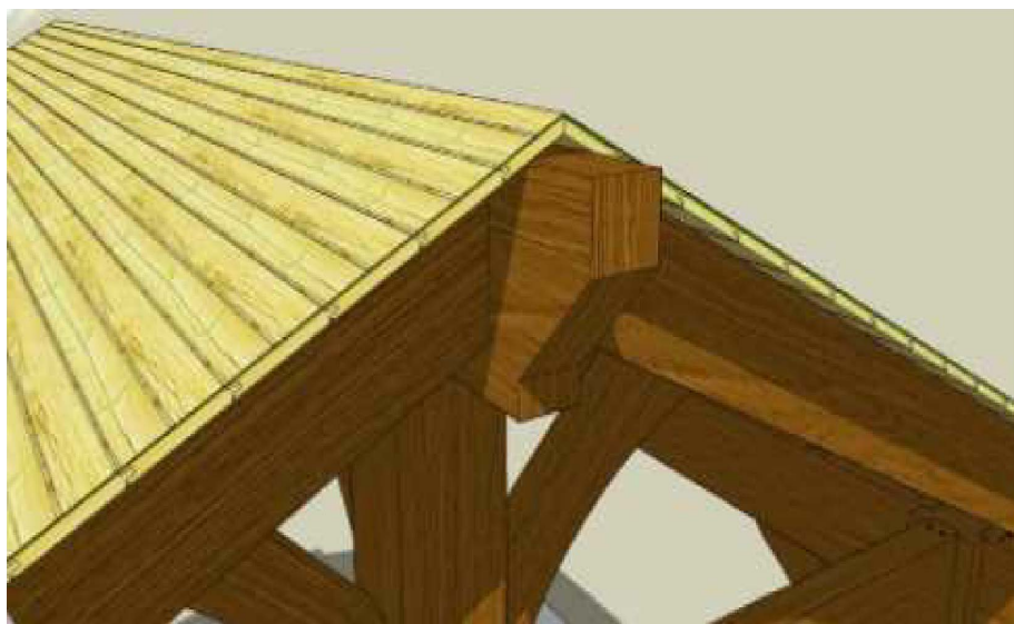
T&G ROOFING MATERIAL (1x6 or 2x6) N.T.S.
