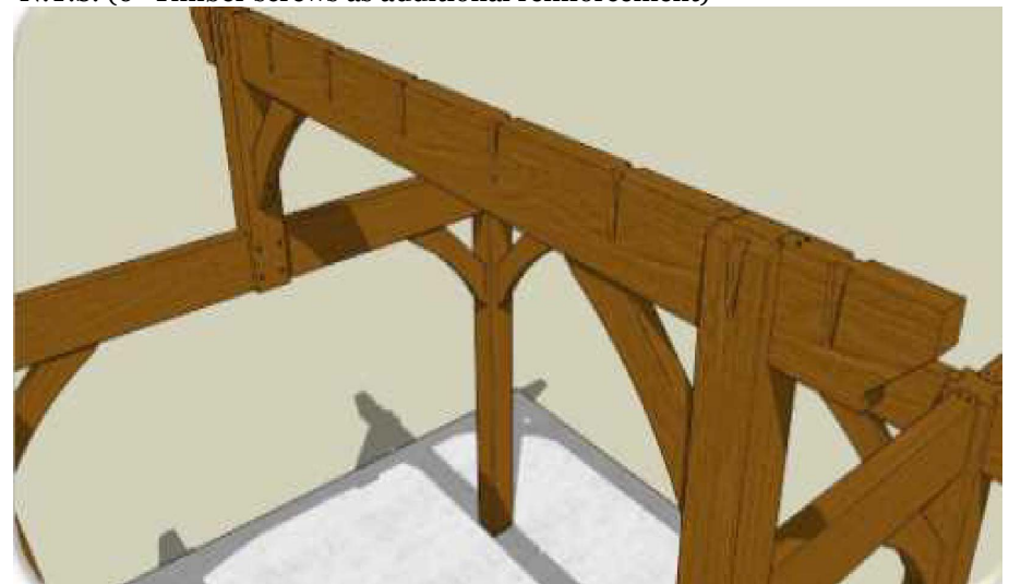
KING POST/RIDGE BEAM CONNECTION (DOVETAIL CONNECTION) N.T.S.
