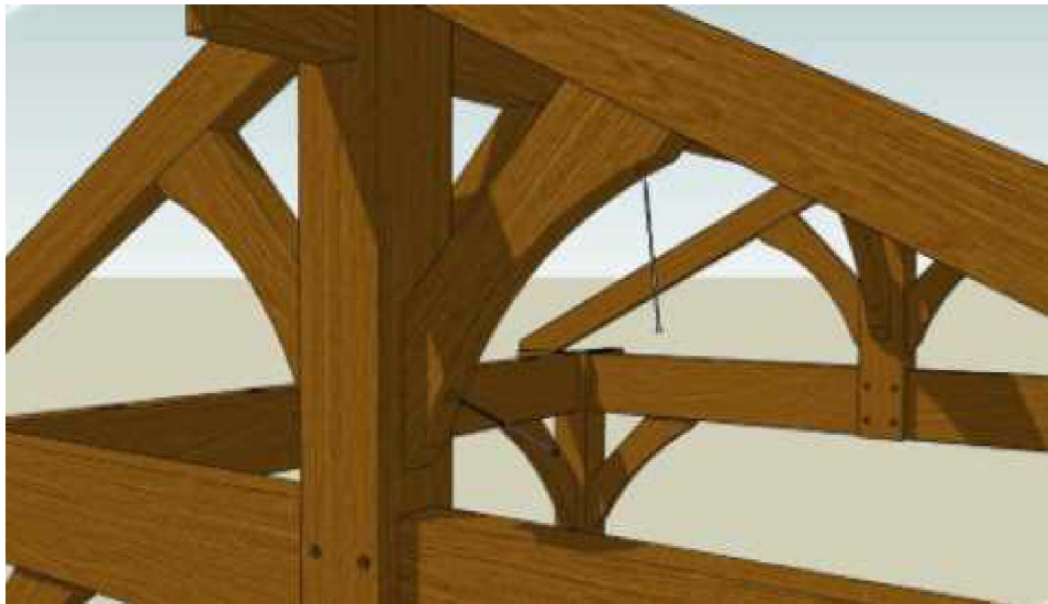
QUEEN BRACES/QUEEN RAFTER CONNECTION N.T.S. (11" timber screw threw queen brace to king post)
