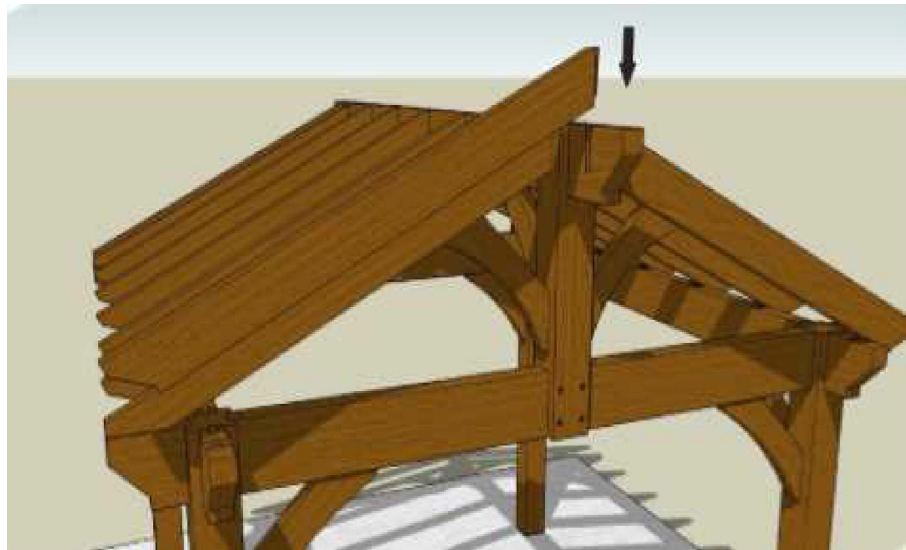
RAFTERS/RIDGE BEAM CONNECTION (DOVETAIL CONNECTION) N.T.S.
