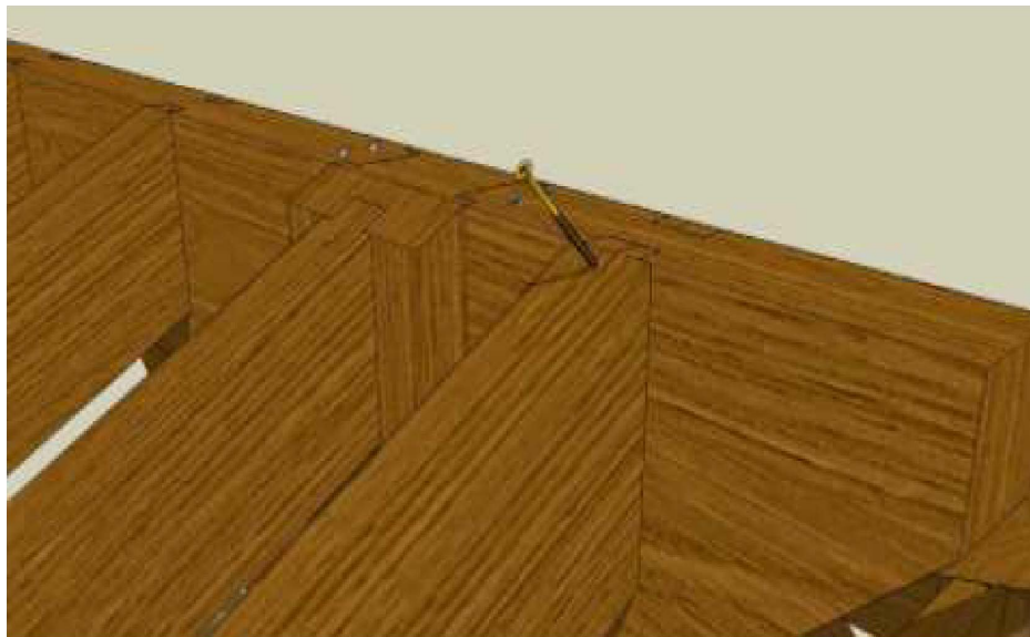
RIDGE BEAM OVERHANG/RAFTER CONNECTION N.T.S. (6" timber screw for additional reinforcement)
