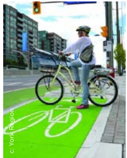
Figure 2.28. Left turn bike box is an example of preventing conflicts arising from bicyclists queuing in a bike lane or a crosswalk.
