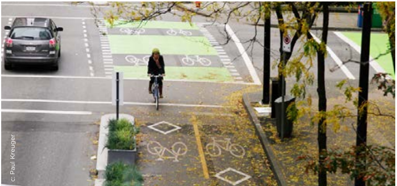
Figure 4.13. Separated bike lanes provide better protection to cyclists.
