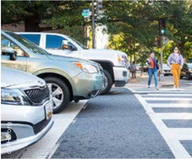
Figure 4.82. Large design vehicles encroaching on space between stop line and crosswalk.
