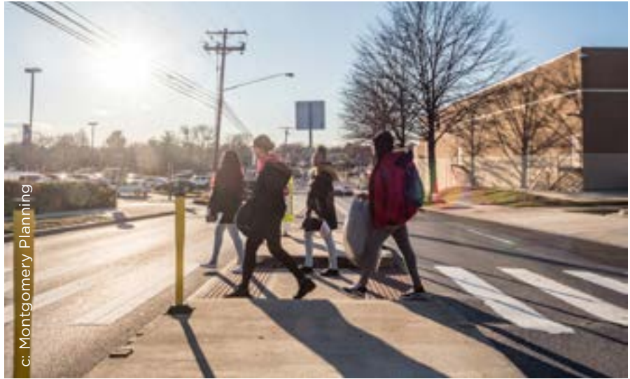
Figure 4.68. Pedestrian refuge with vertical elements and signage.
