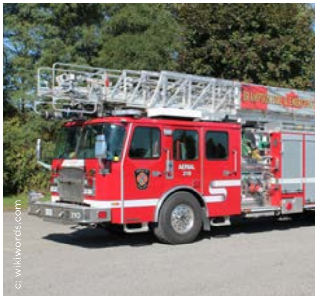
Figure 2.16. Control vehicles, like fire trucks, are the largest vehicles that use city streets. They are permitted to use more of the street to manoeuvre.
