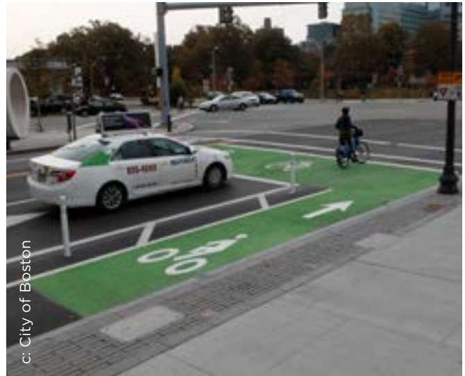
Figure 4.83. Advanced stop lines accommodate bike boxes at intersection.
