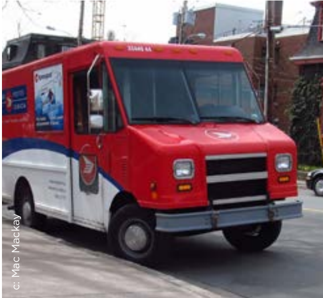
Figure 2.15. Design vehicles are the most common large vehicles that use city streets, similar to a Canada Post or other courier trucks.
