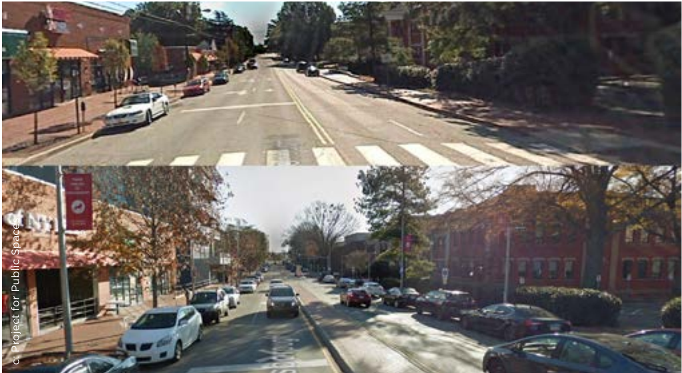
Figure 4.19. Right-sizing Hillsborough Street (City of Raleigh, NC) resulted in a 23% decrease in vehicle crashes. It involved reducing four travel lanes to two, adding on-street parking, bike lanes and a median, and widening sidewalks.
