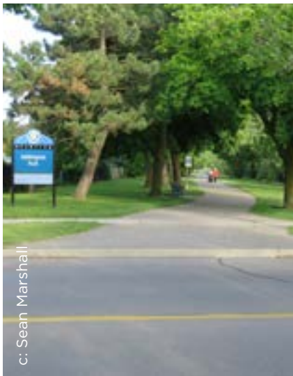
Figure 2.26. Missing crosswalks when recreational trails meet major roads.
