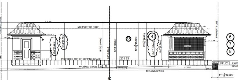
PROPOSED ELEVATION AT REAR OF PROPERTY TO DEMONSTRATE RATIONAL OF RETAINING WALL AND CABANA HEIGHT IN RELATION TO GRADES FROM PROPERTY LINE TO PROPERTY LINE
