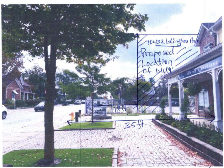
Proposed building to sidewalk 18ft. (5.5m) Adjacent building to sidewalk 35ft (10.7m)
