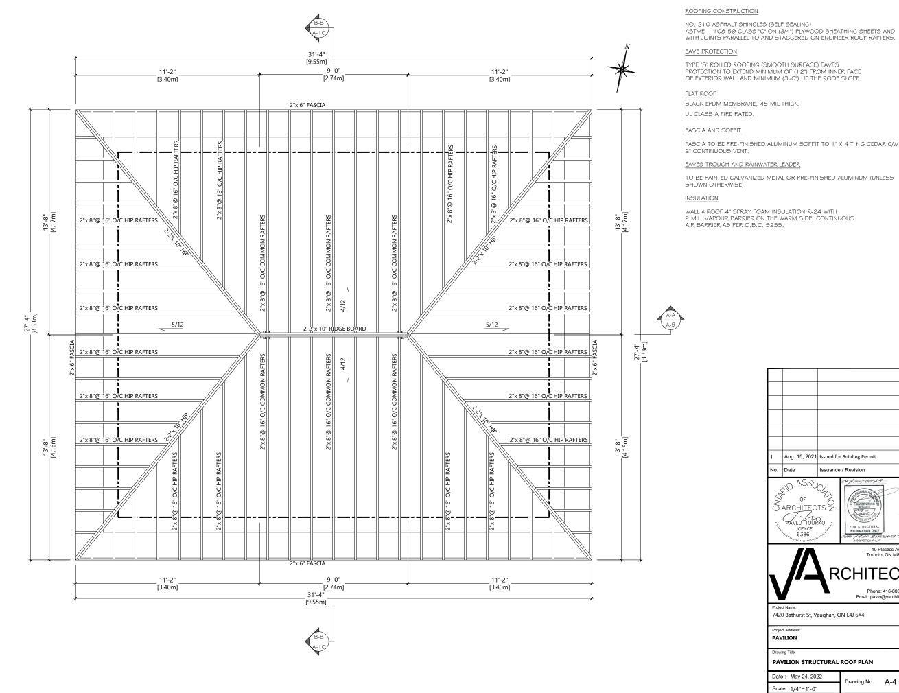
TYPE "S" ROLLED ROOFING (SMOOTH SURFACE) EAVES PROTECTION TO EXTEND MINIMUM OF (12") FROM INNER FACE
