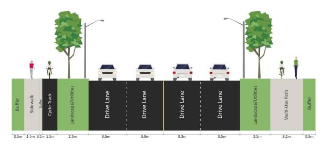
**Note**: This alternative considers implementation of MUP(s) and/or side-by-side facilities (both are illustrated in the above cross-section as an example)
