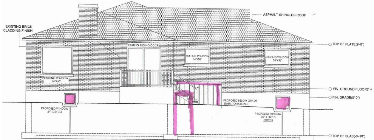
East Elevation, new window opening and below grade stair, not visible from the street.
