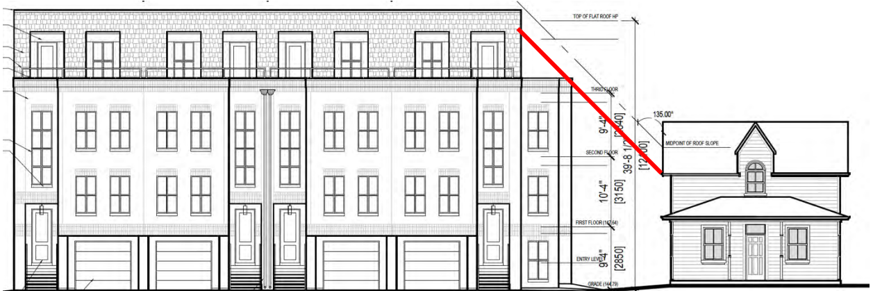
BLOCK B ELEVATION – transition in height to the 1.5 storey adjacent contributing building at 148 Wallace Street that maintains a 45 degree angle
