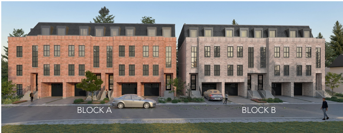
WALLACE STREET ELEVATION – two blocks of 3.5 storey townhouses with four units in each block. Block A is clad with red brick. Block B is clad with buff brick. The roof form is mansard roof with dark metal cladding.
