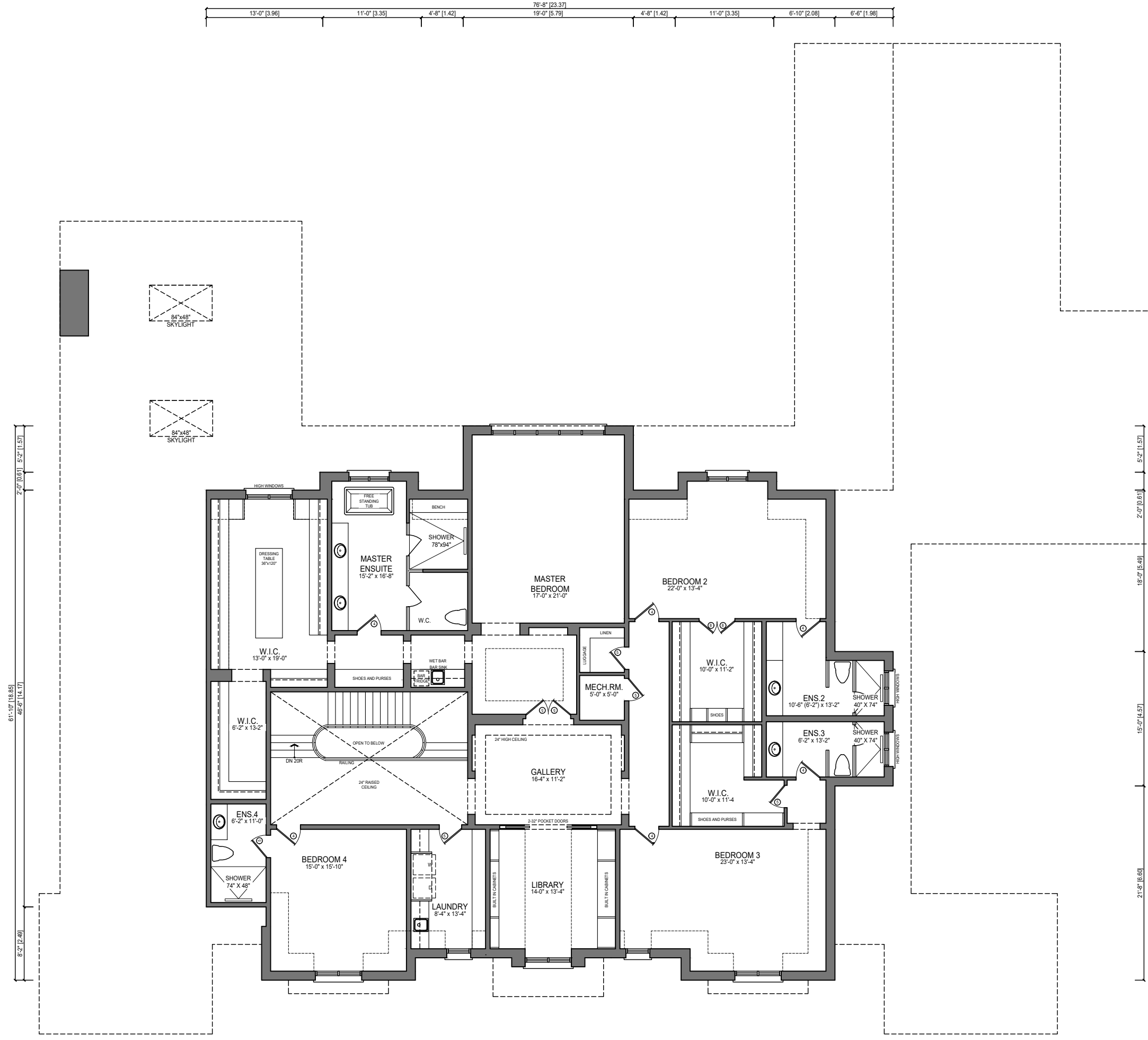
SECOND FLOOR PLAN SECOND FLOOR AREA = 3996 sq. ft. OPEN TO BELOW (inc.) = 38 sq. ft.
