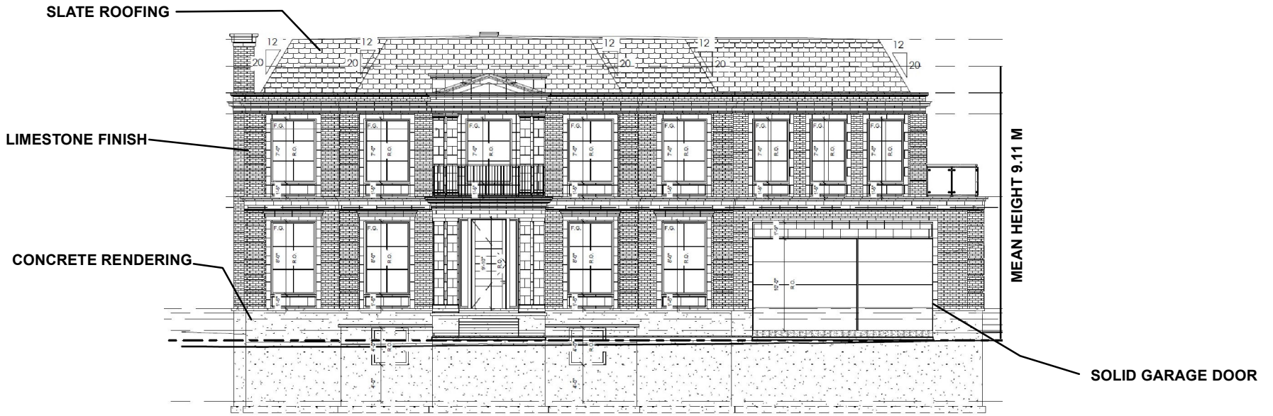
DWELLING B - EAST ELEVATION (FRONT)
