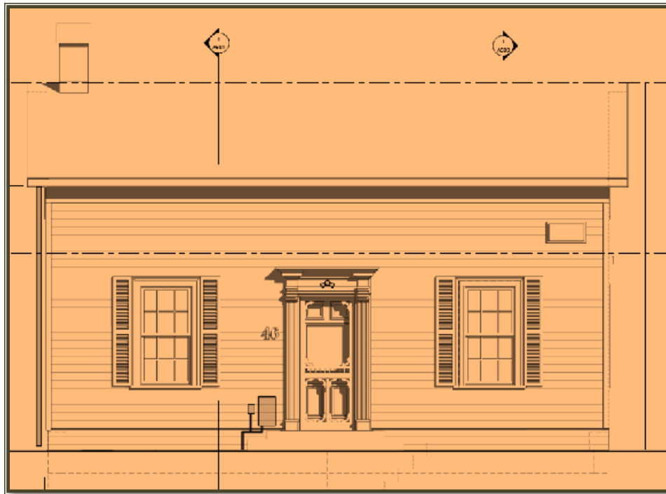
5.3.2 Measured drawing of front elevation showing the symmetrical facade with well-detailed classical door surround, courtesy Phaedrus Studio, 1 August 2017.
