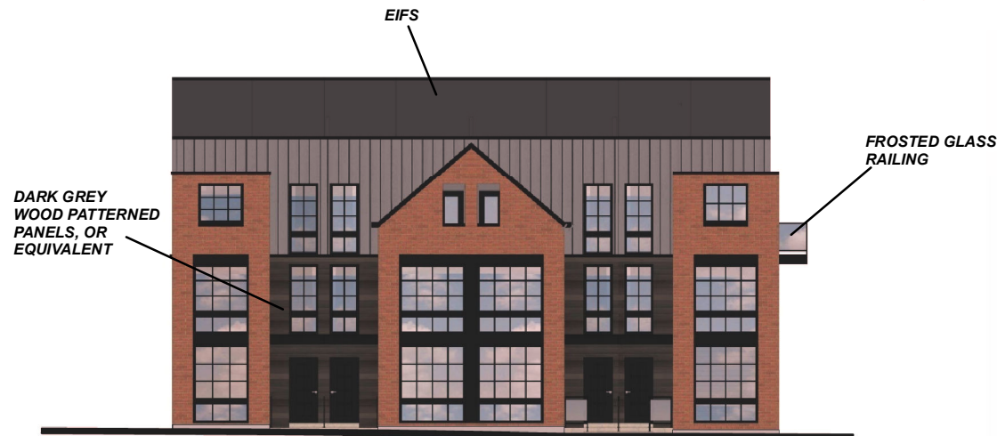
BLOCK 12 WEST ELEVATION
