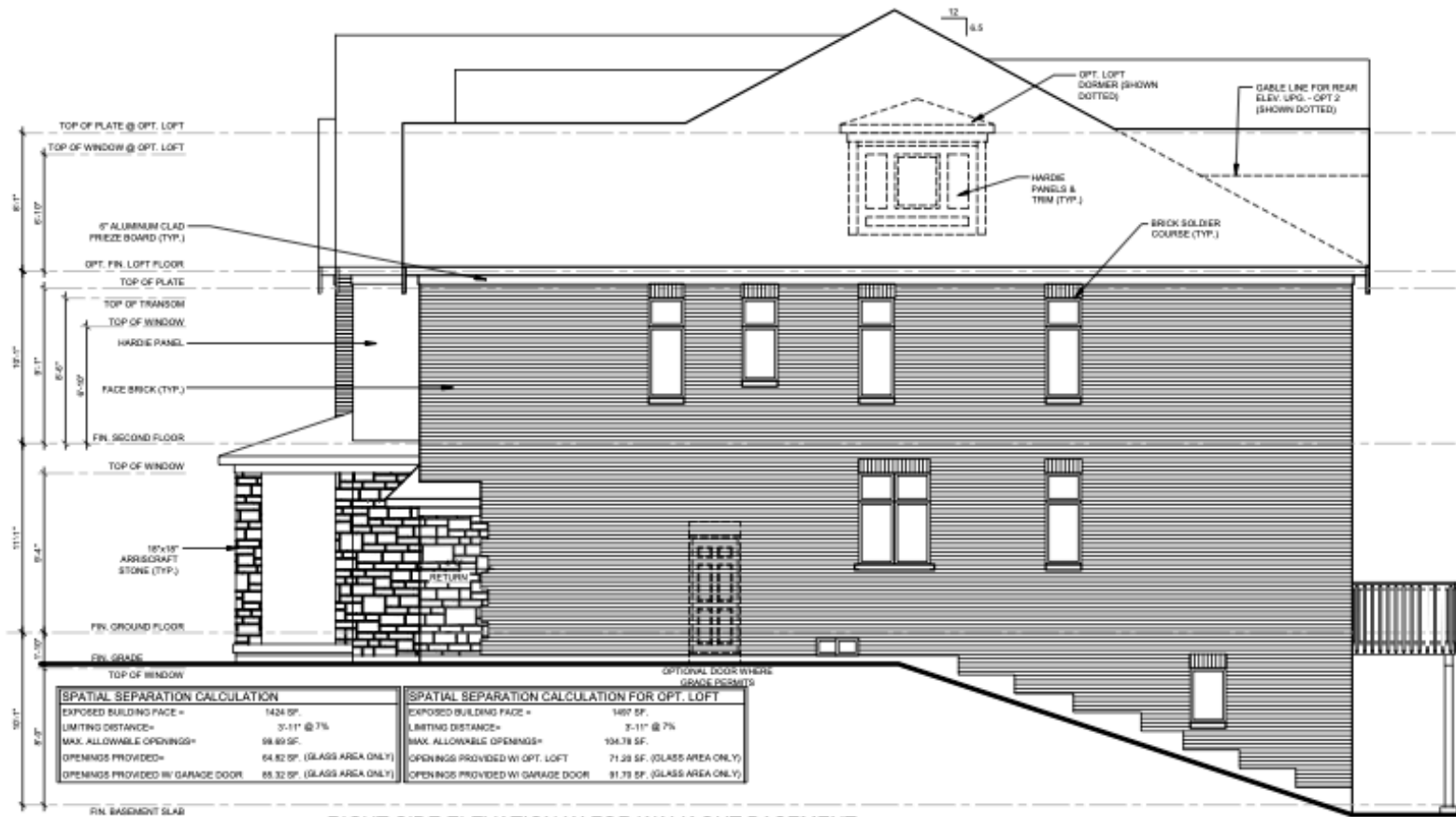
RIGHT SIDE ELEVATION 'A' FOR WALK OUT BASEMENT WITH REAR ELEVATION UPGRADE FOR OPT. 1 OR OPT. 2
