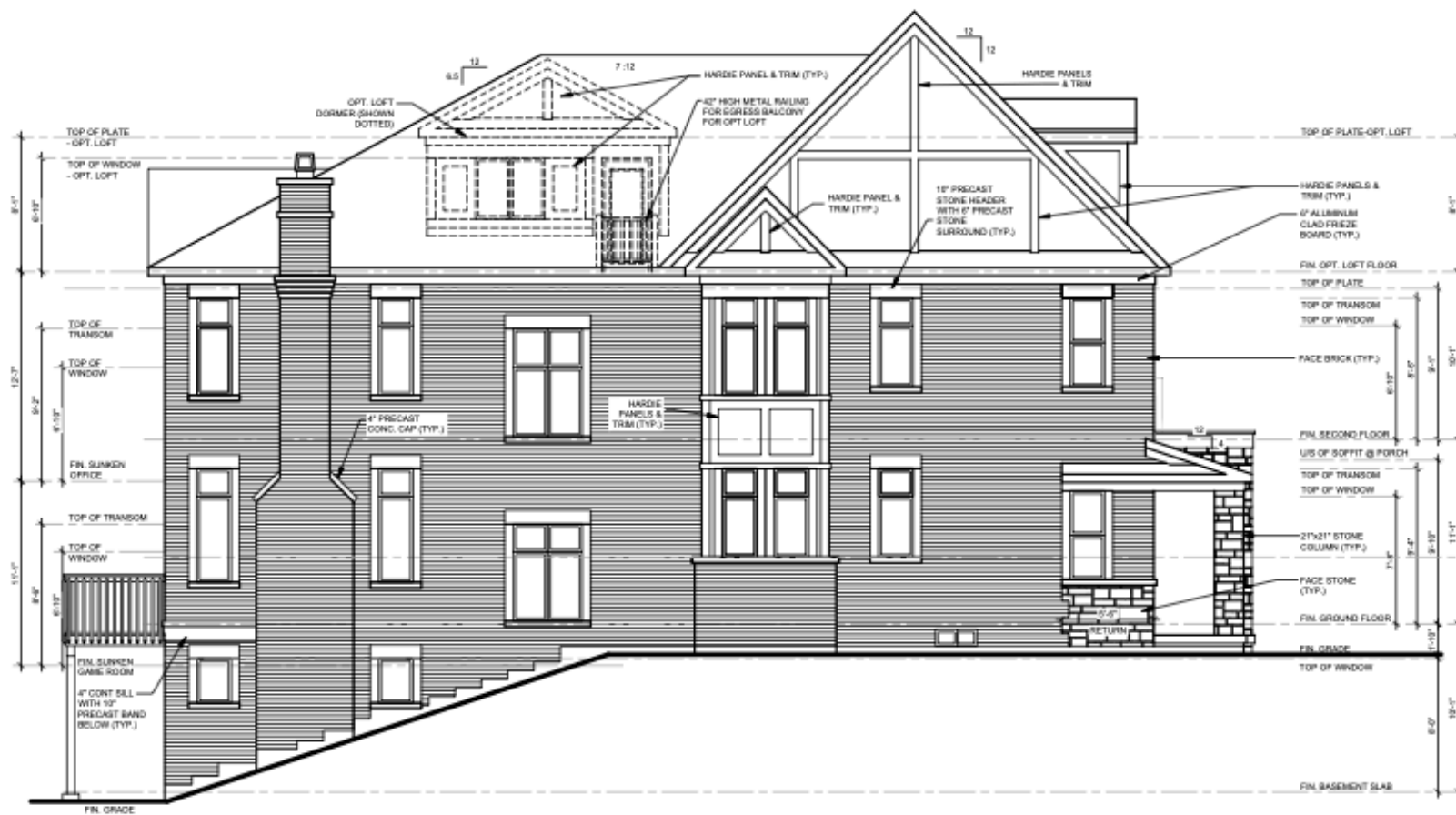
50-3 UNITS 1 AND 13 LEFT SIDE UPGRADE ELEVATION 'C' FOR WALK OUT BASEMENT - OPT.1 WITH REAR ELEVATION UPGRADE FOR OPT. 1
