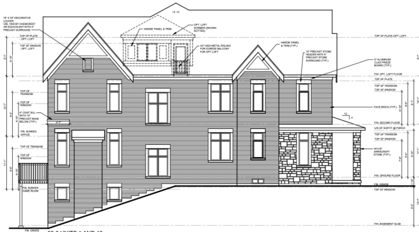
50-3 UNITS 1 AND 13 LEFT SIDE UPGRADE ELEVATION 'A' FOR WALK OUT BASEMENT - OPT.2 WITH REAR ELEVATION UPGRADE FOR OPT. 2
