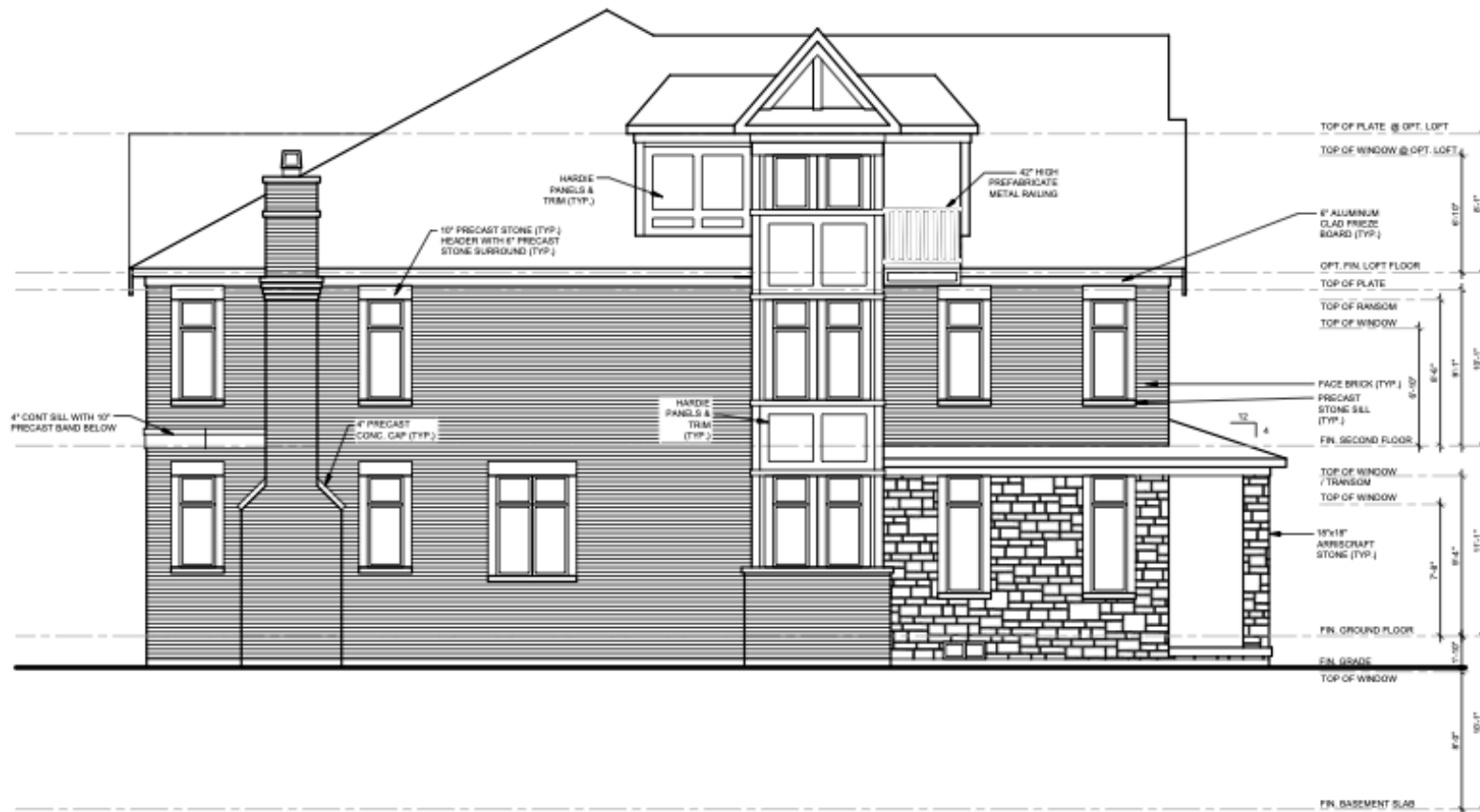
50-2 UNITS 1 AND 13 LEFT SIDE UPGRADE ELEVATION 'A' - OPT. 2 W/ OPT. LOFT
