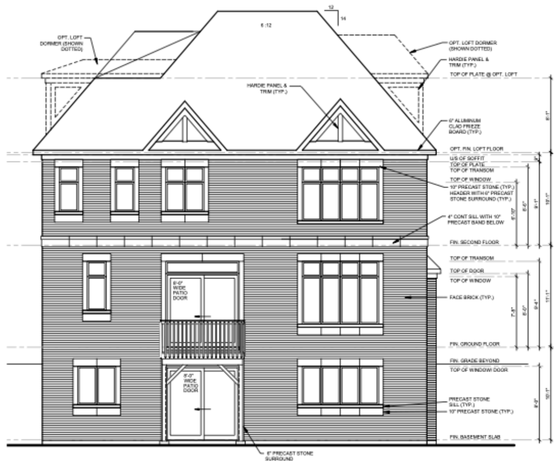
REAR ELEVATION 'D' FOR WALK OUT BASEMENT UPGRADE OPTION 2
