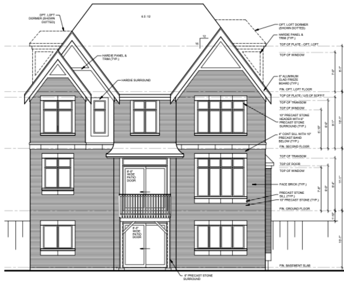
REAR ELEVATION 'E' FOR WALK OUT BASEMENT UPGRADE OPTION 1
