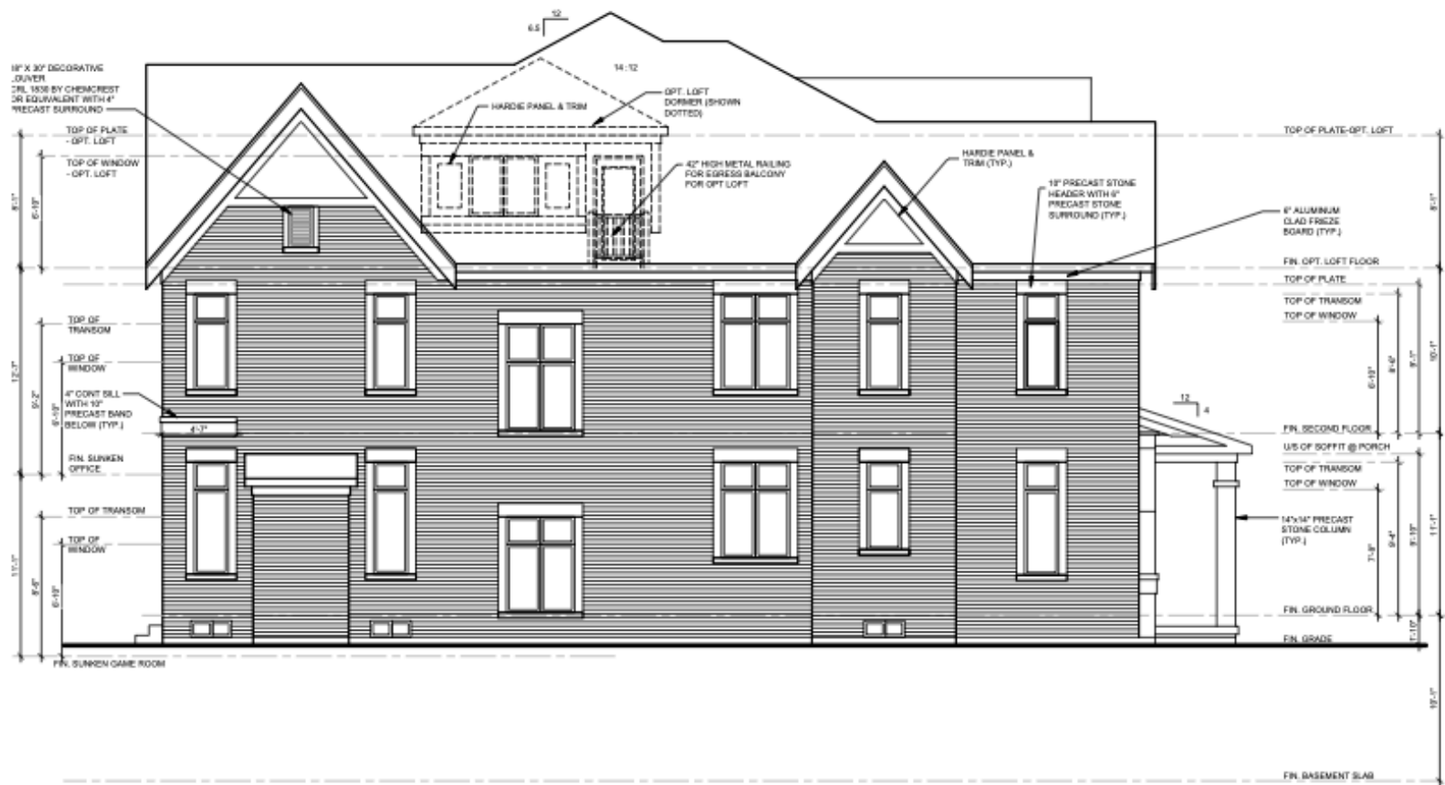
50-3 UNITS 1 AND 13 LEFT SIDE UPGRADE ELEVATION 'B' - OPT. 2
