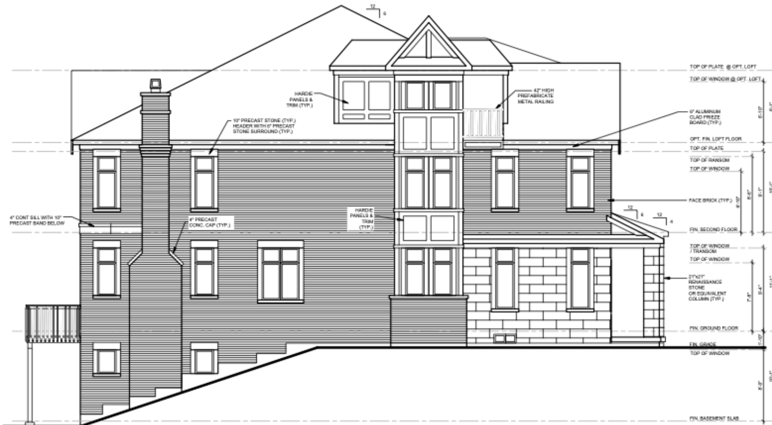
50-2 UNITS 1 AND 13 LEFT SIDE UPGRADE ELEVATION 'D' FOR WALK OUT BASEMENT - OPT.2 WITH REAR ELEVATION UPGRADE OPTION 2 & OPT. LOFT
