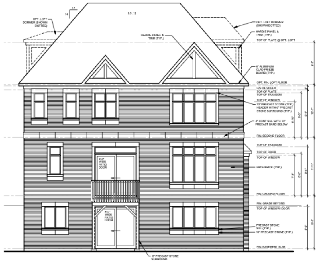
REAR ELEVATION 'B' FOR WALK OUT BASEMENT UPGRADE OPTION 2
