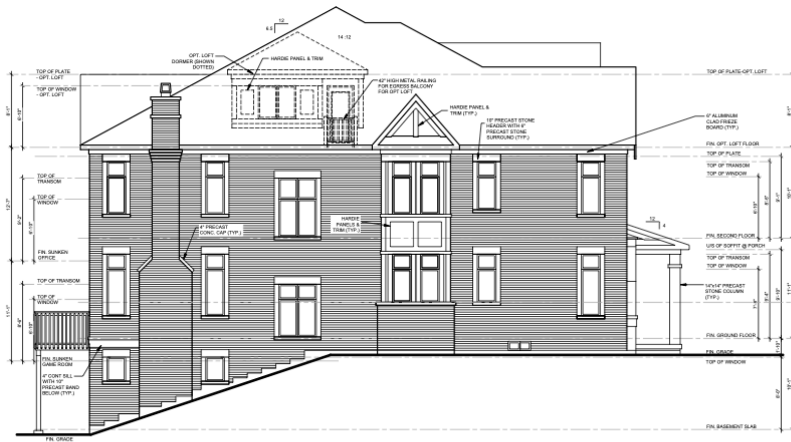
50-3 UNITS 1 AND 13 LEFT SIDE UPGRADE ELEVATION 'B' FOR WALK OUT BASEMENT - OPT.1 WITH REAR ELEVATION UPGRADE FOR OPT. 1
