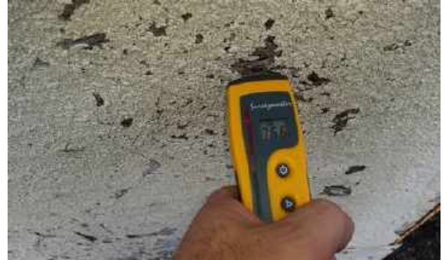
Water saturated stucco wall
