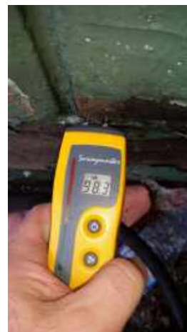
Water saturated block wall.
