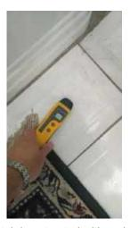
Tile floor near tub is saturated with moisture.
