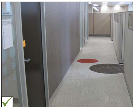
Examples of floor surface and elevator door finishes that minimize glare.
