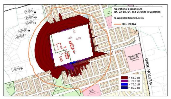
Produced by Stantec on behalf of TCPL. Contours based on several assumptions including absorption coefficients for the building facades that corresponded to brick (or brick veneer) with 10-mm pointing (mortar recess). The model groups individual buildings as single structures and acoustic transparency has been assigned to the structures representing groups of buildings to account for passages between the individual buildings.
