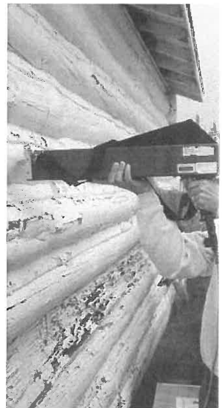
Using minimally destructive testing methods can help evaluate the condition of wood without damaging it. Here a resistance measuring micro drill is being used to evaluate the condition of a log wall at Fort Walsh, NHSC in Saskatchewan. A drilling needle penetrates the wood at a constant speed and measures the resistance encountered to advance the drill bit. The resistance the wood offers indicates its condition: low resistance can indicate decay.
