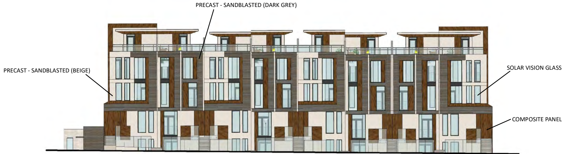
TYPICAL STACKED TOWNHOUSE ELEVATION (BLOCK 2 - FACING SOUTH)
